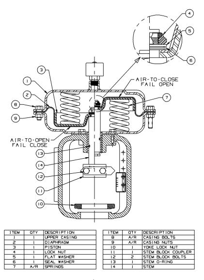
Figure 1 – AutoSeal Actuator Section View
